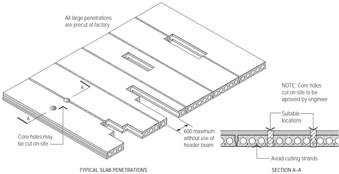
**Figure 19** Penetration Positions
