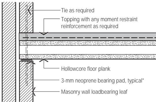
EXTERNAL MASONRY CAVITY WALL DETAIL
