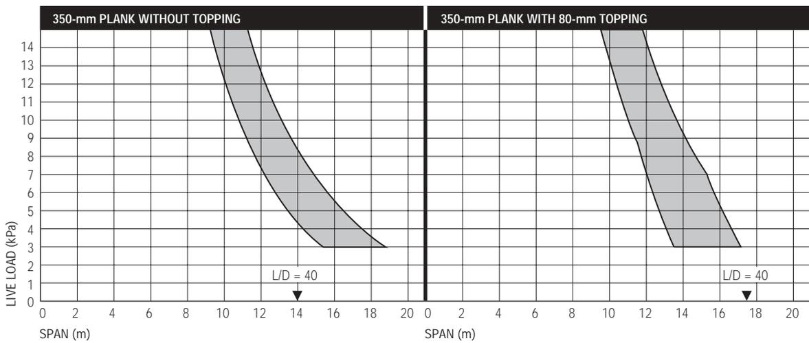
**Figure 6** 350-mm Hollowcore Planks – Live Load Capacity
