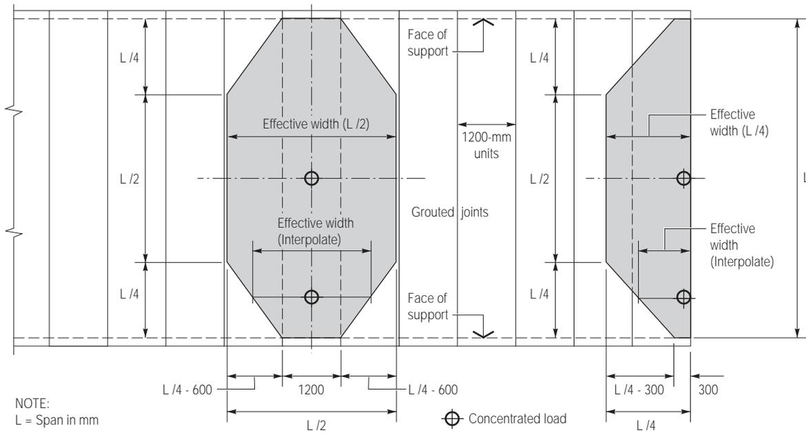
**Figure 8** Linear Load Distribution of Concentrated Loads (PCI)
