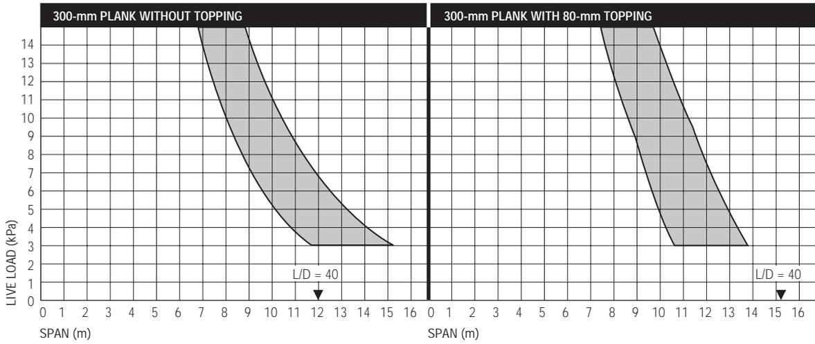
**Figure 5** 300-mm Hollowcore Planks – Live Load Capacity
