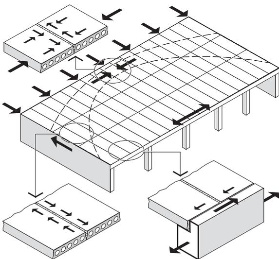
**Figure 14** Horizontal Load Transfer by Diaphragm Action
