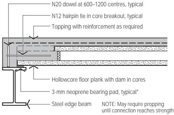
EXTERNAL STEEL BEAM DETAIL
