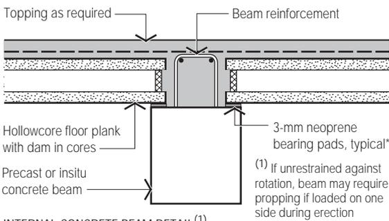
INTERNAL CONCRETE BEAM DETAIL<sup>(1)</sup>
