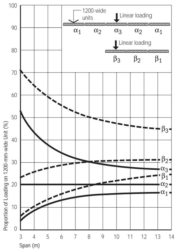
**Figure 9** Load Distribution Coefficients – Centrally-Placed Line Load (FIP)
