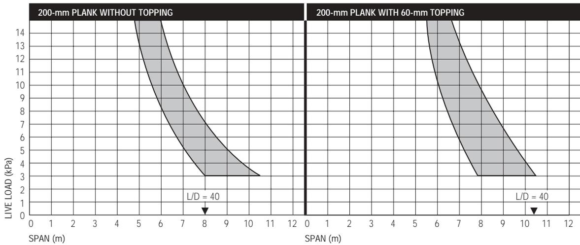
**Figure 3** 200-mm Hollowcore Planks – Live Load Capacity
