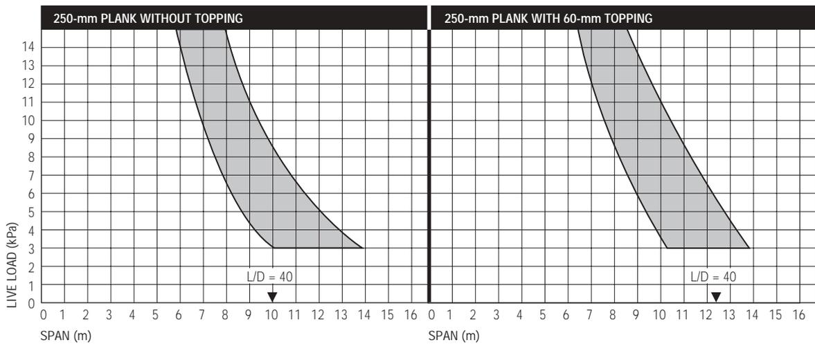
**Figure 4** 250-mm Hollowcore Planks – Live Load Capacity
