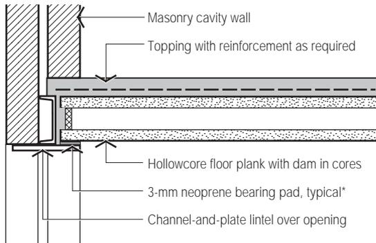
EXTERNAL CHANNEL-AND-PLATE LINTEL DETAIL
