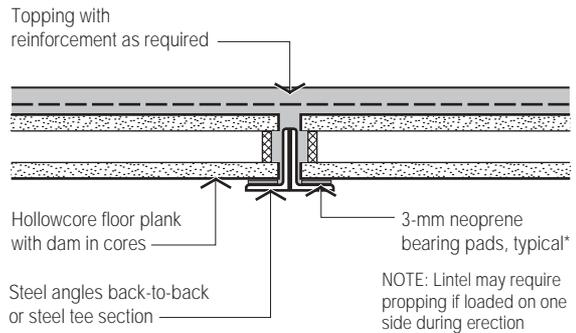
INTERNAL ANGLE OR TEE LINTEL DETAIL
