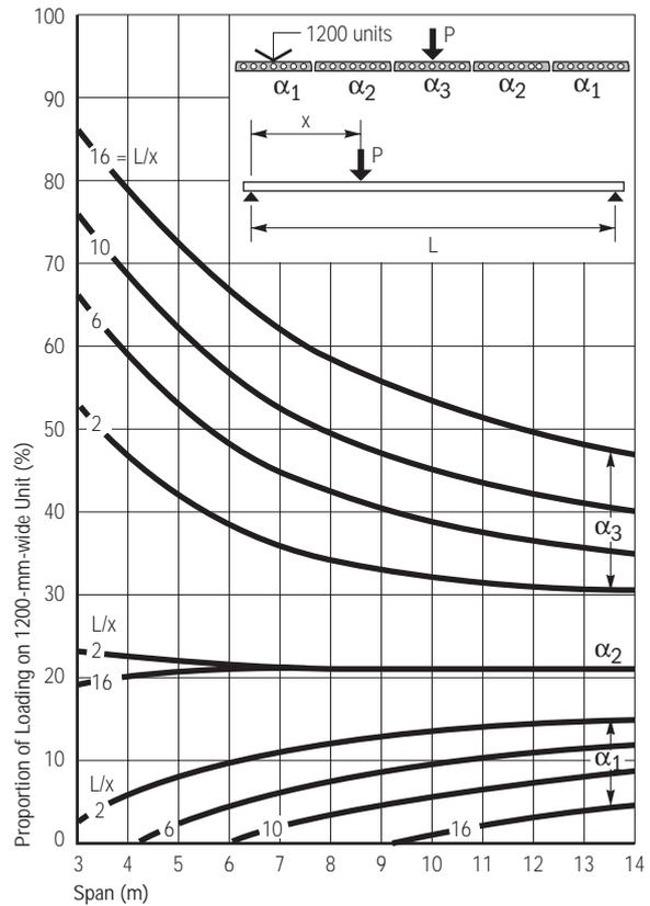
**Figure 10** Load Distribution Coefficients – Point Load (FIP)
