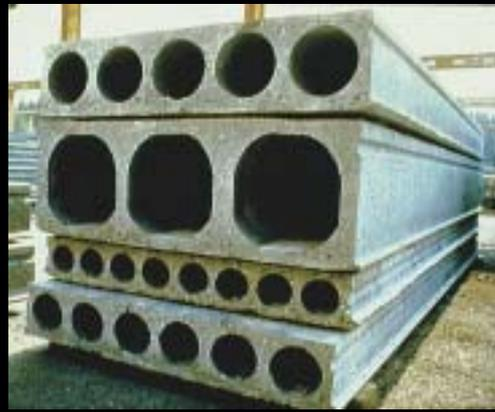
*Hollowcore units are machine-made in a factory. They are nominally 1200 mm wide, range in thickness from 150 mm to 400 mm and come with a variety of core configurations depending on the type of production equipment*
