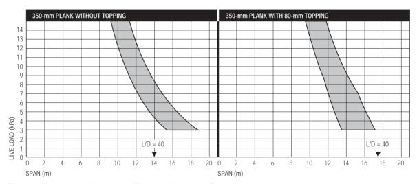
Figure 6 350-mm Hollowcore Planks – Live Load Capacity
