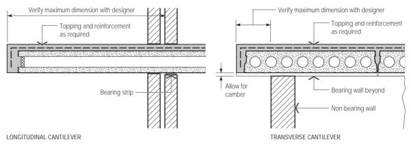
Figure 12 Longitudinal and Transverse Cantilever Arrangements
