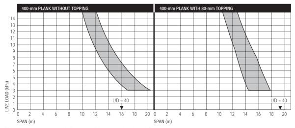
Figure 7 400-mm Hollowcore Planks – Live Load Capacity
