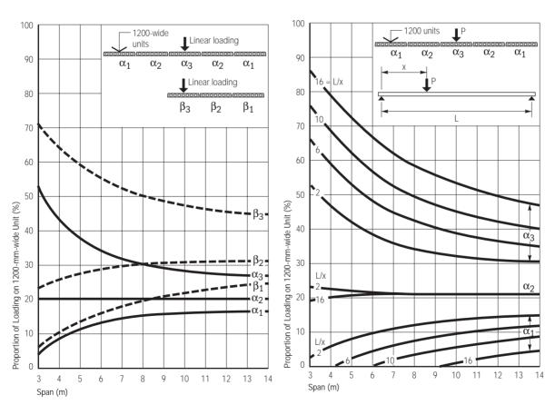
Figure 9 Load Distribution Coefficients – Centrally-Placed Line Load (FIP)
