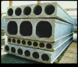
Hollowcore units are machine-made in a factory. They are nominally 1200 mm wide, range in thickness from 150 mm to 400 mm and come with a variety of core configurations depending on the type of production equipment
