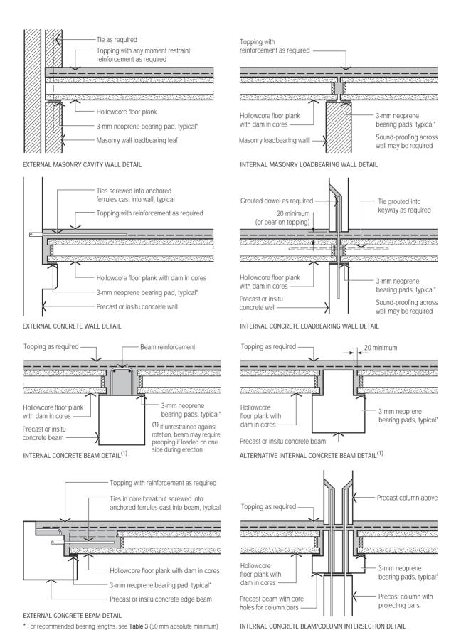
Figure 16 Concrete and Masonry Bearing Support Details
