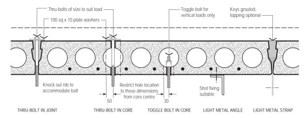
Figure 21 Typical load hangers
