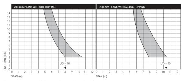
Figure 3 200-mm Hollowcore Planks – Live Load Capacity
