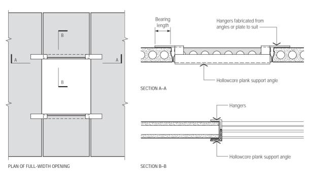
Figure 20 Typical Header Arrangement
