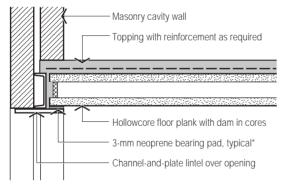
EXTERNAL CHANNEL-AND-PLATE LINTEL DETAIL
