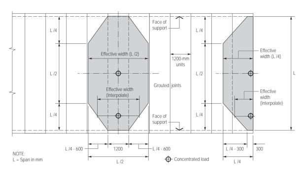
Figure 8 Linear Load Distribution of Concentrated Loads (PCI)
