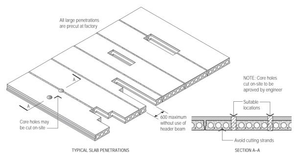
Figure 19 Penetration Positions
