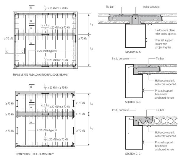
Figure 13 Minimum tensile Capacities of Integrity Ties [After Item 3, Chapter 8]
