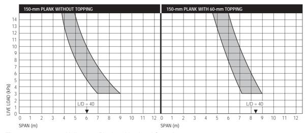
Figure 2 150-mm Hollowcore Planks – Live Load Capacity
